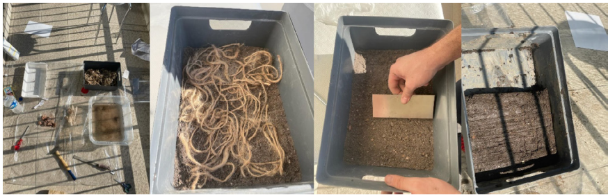
Figure 2: Production process of Adobe-Hemp prescriptions
