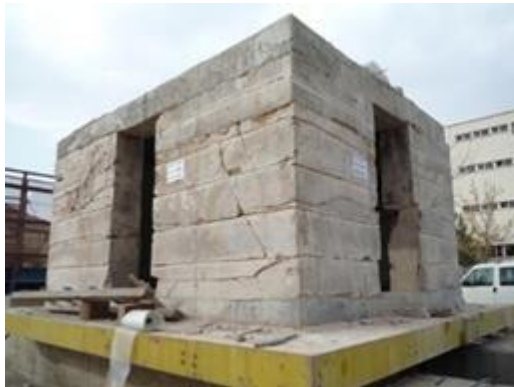
Figure 2 a. Condition of Masonry Building After Earthquake Applied 8 Times [3]; Figure b. Creating a fracture plane [4]
