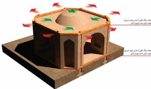
Figure 9. Simulation of lateral load path
