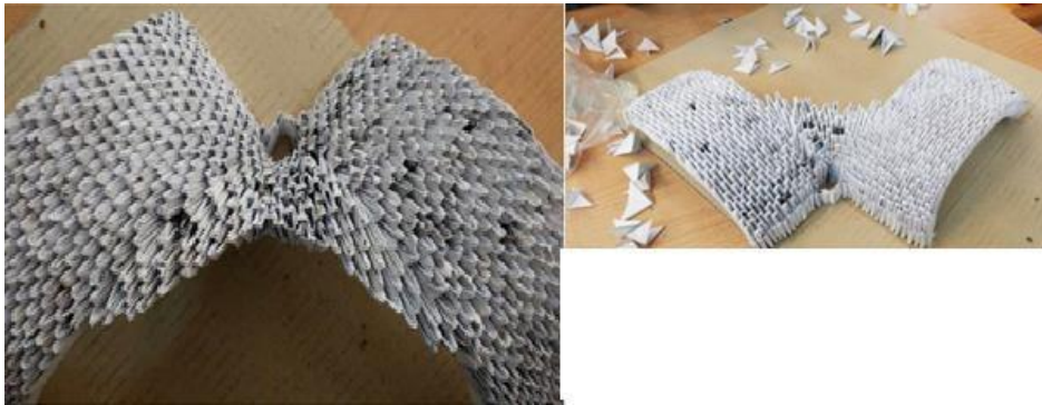
Figure 2. Exercise 1, design and construction of a maquette of a compression structure by students who used paper and origami techniques to show how compressive forces are transferred. More than a thousand paper pieces are used in this maquette as compressive elements.
