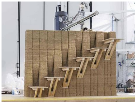
Figure 4. 3D printing adobe wall with built-in staircase [25].
