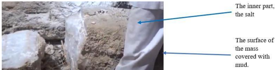
Figure 5. The Salt rocks after extracting and preparing for cutting and cleaning, Siwa Oasis-Egypt (URL1, video)
