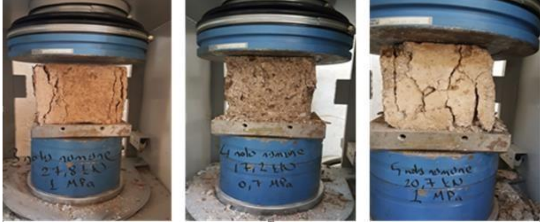
Figure 5. E1 soil sample (in the middle) was tested for compressive strength and passed, Erzincan Binali Yıldırım University, 22 October 2020.
