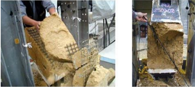
Figure 3 a, Example of unbroken Wall b. Diagonal crack formation [6]
