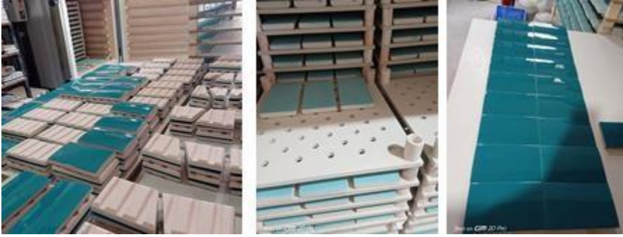
Figure 17. The tiles are in to the kiln (Resource: Personal Archive); Figure 18, The tiles are cooling (Resource: Personal Archive); Figure 19. The tiles are ready to use (Resource: Personal Archive)
