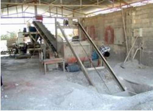
Figure 17. Concrete paving stone machine, used for 60 000 earth block production; Figure 18. URFA- GAP four official residence, 400 m2, earth block construction at 2000
