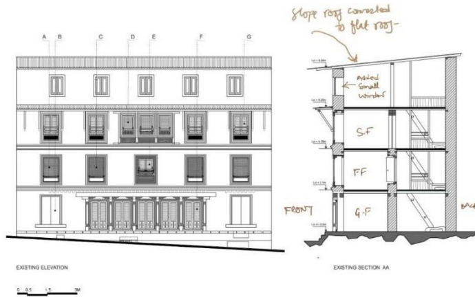
Figure 8. Elevation and section of observed changes in roof and attic wall in the traditional building.
