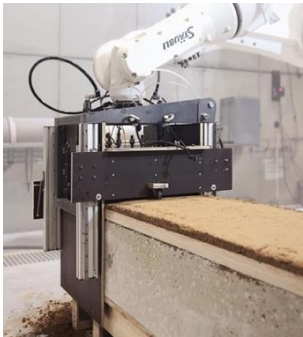
Figure 5. Robotic rammed earth production [27].
