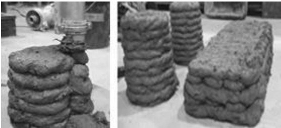
Figure 6. 3D printed cob cylinders’ production from a robot arm.
