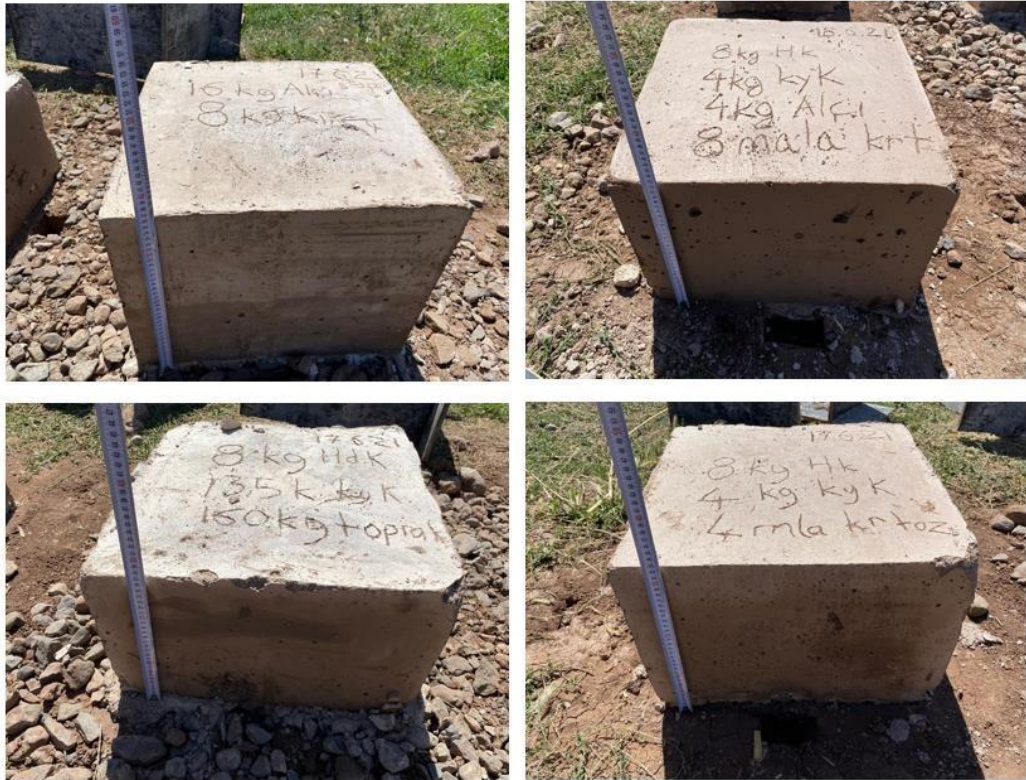
Figure 11. Soil mixture samples at different ratios were prepared and poured into the mold, 20 June 2021
